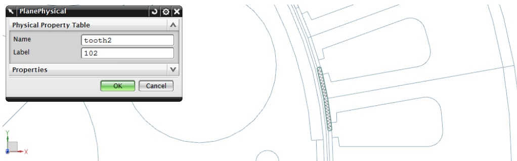
Picture: Faces in the Air Gap on which Forces are computed
